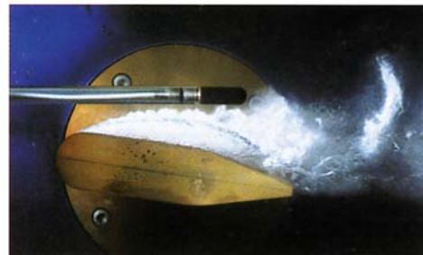
Fig. 10 Appearance of cloud cavitation (KT section, \alpha = 8 deg, U_\infty = 12 m/s, \sigma = 1.25 )
